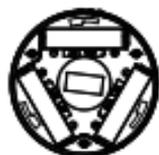
3. Close the hatch cover by turning clockwise according to the marking.
